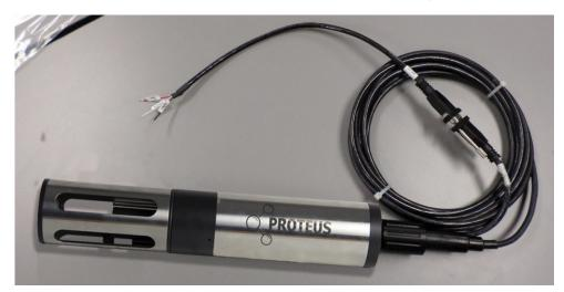
If you wish to retrofit a Proteus with the MIB option, please contact us. If you wish to build your own MODBUS or SDI-12 converter cable, or convert your Underwater Cable into a converter cable, use the wiring diagrams in Appendices One and Two.
