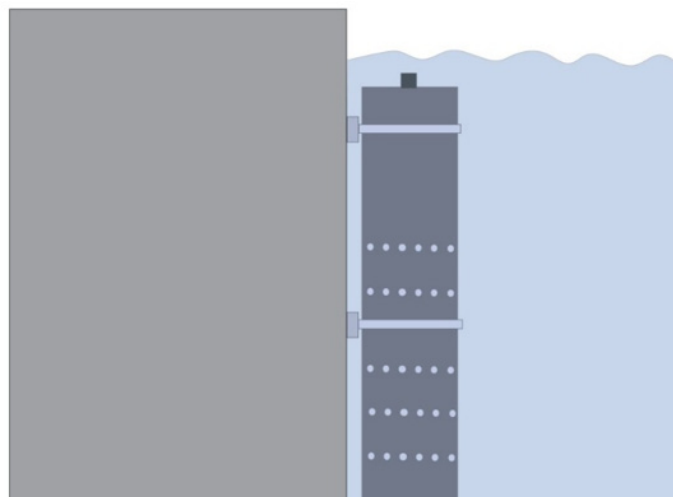
Figure 20: Installation of Proteus in perforated stilling tube.
