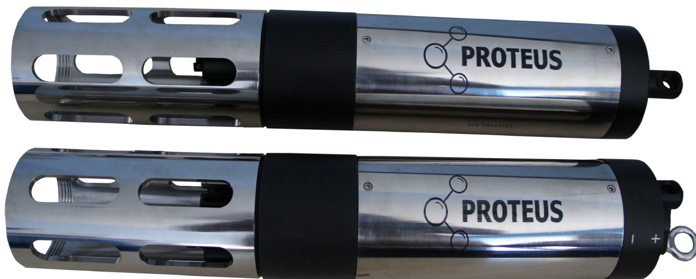
Figure 6: Direct comparison of Proteus with IBP (foreground) and Proteus without IBP (Background).
