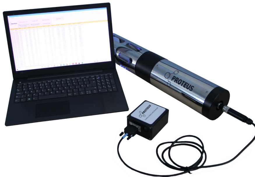
Figure 38: Proteus connected via BBP to a Bluetooth enabled laptop.
