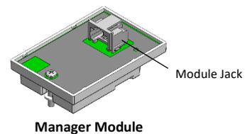
The RXW Manager consists of a mote with a cable attached that is plugged into a module, which is installed in the RX3000 station. These are the components of the mote and module.
