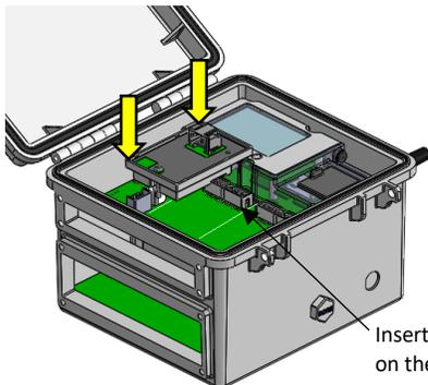
Insert the connectors on the module here
