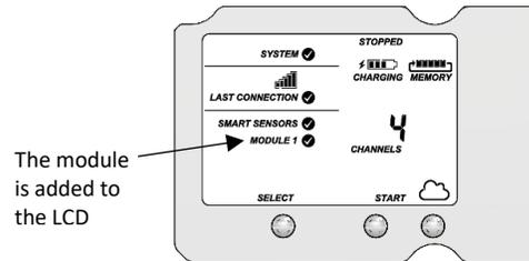
The module is added to the LCD
