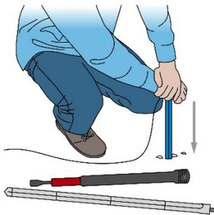
8. Once the probe is fully inserted in the hole, pack the soil around the top of the sensor to prevent water from
