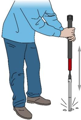
5. Once the pilot rod reaches the desired depth, extract the pilot rod by using the slide hammer in reverse, lifting it rapidly to hammer upwards. Be sure to hold the slide hammer vertically without side-to-side movement to extract the pilot rod straight up.
