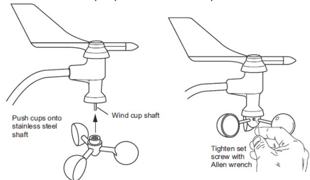
3. Use the Allen wrench provided to tighten the set screw on the side of the wind cups. The wind cups should drop slightly when you let go.
