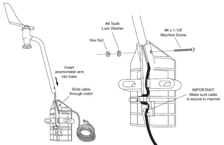
2. Insert the machine screw through the holes in the base and arm.
