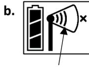
b. Once a network is found, the icon will stop flashing and the bars will cycle from left to right.
