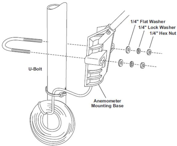
2. Raise the anemometer to the desired height on the pole and swivel it so the anemometer arm is pointing north.
