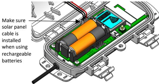
The mote contacts the network once the new batteries are installed. The green LED blinks quickly while the mote searches for a network to join and then blinks slowly while it completes the network registration. Once the mote has finished joining the network, the green LED turns off and the blue LED then blinks indefinitely while the mote is part of the network.
