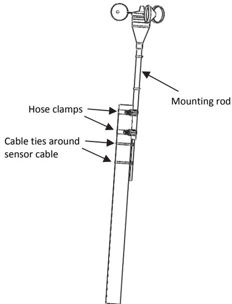
3. Tighten the hose clamps making sure the mounting rod remains vertical.
