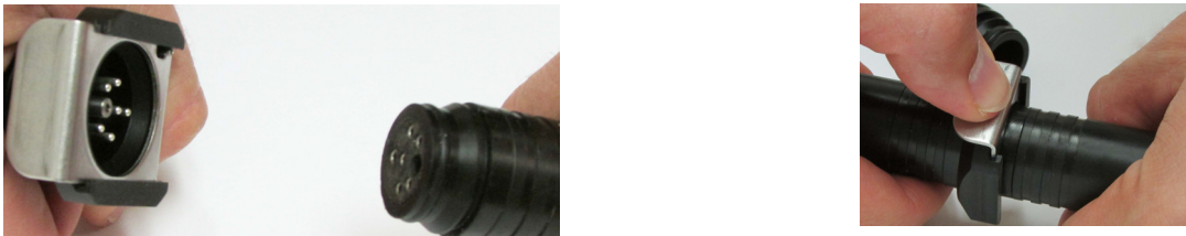
Figure 4-13 How to connect a TIENet receptacle to the Signature Portable
