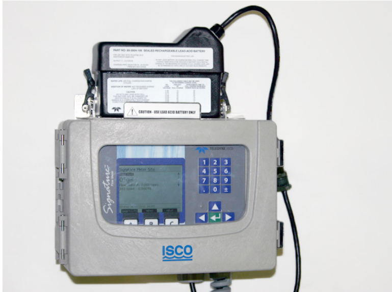
Figure 5-8 Backup battery, installed
