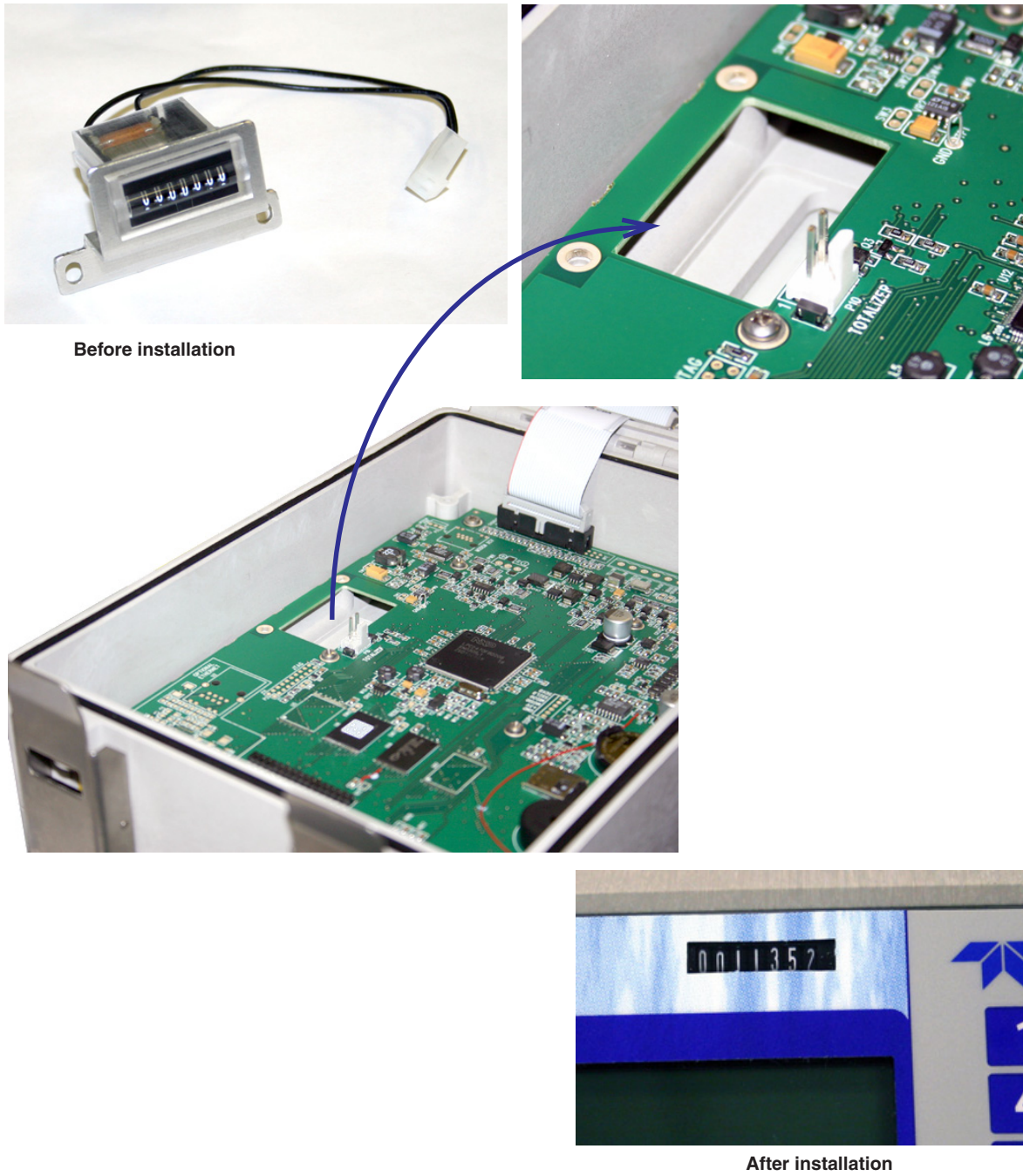
Figure 5-10 Optional non-resettable totalizer installation
