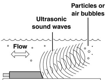
The 350 area velocity sensor contains a pair of ultrasonic transducers. One transducer transmits the ultrasonic sound wave. As the transmitted wave travels through the stream, particles and bubbles carried by the stream reflect the sound wave back at the sensor. The second transducer receives the reflected wave.
