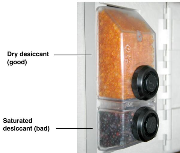
Figure 4-1 Desiccant indicating saturation
