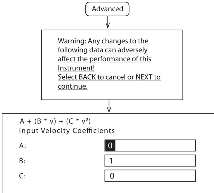
Figure 3-4 Measurement setup: Advanced settings for 350 AV sensor
