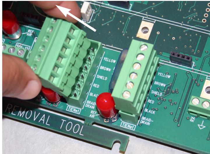
Figure 2-5 TIENet Device terminal strips
