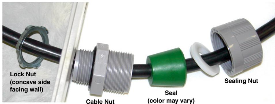
Figure 2-6 Installing cable with a cord-grip fitting
