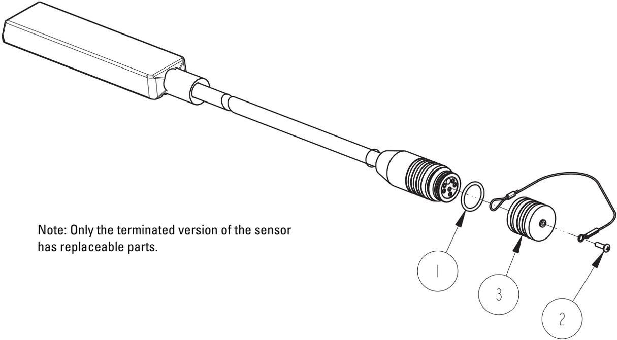
Note: Only the terminated version of the sensor has replaceable parts.
