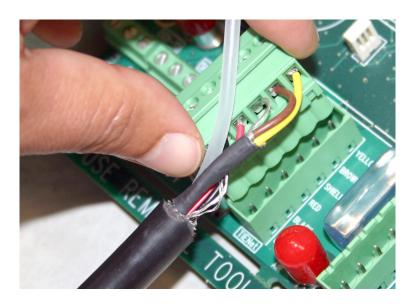
Figure 2-8 Attach wired terminal strip to case board socket
