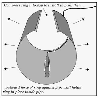
Figure 2-11 Sensor Installed on a Spring Ring
