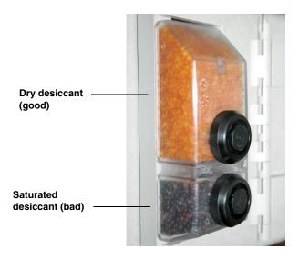
Figure 4-1 Desiccant indicating saturation
