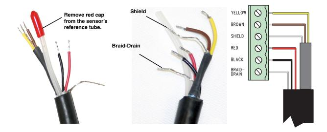
Figure 2-7 TIENet Device terminal connections
