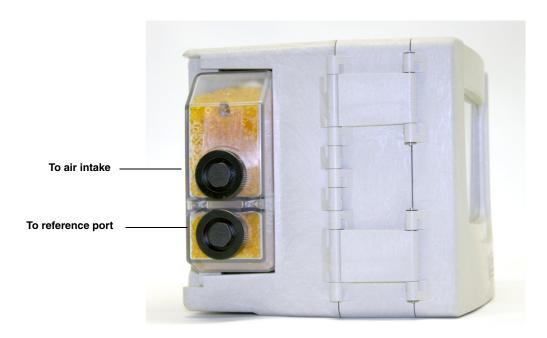
Figure 2-3 External desiccator, installed
