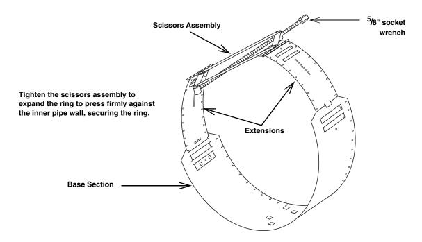
Figure 2-12 Scissors Ring adjustment
