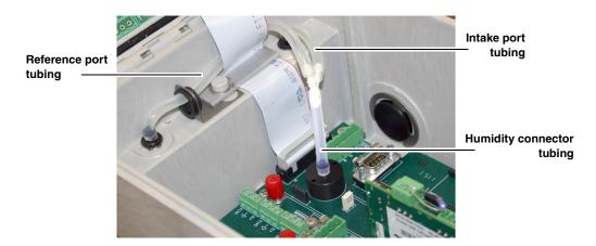
Figure 2-4 Tubing configuration for optimal drying power
