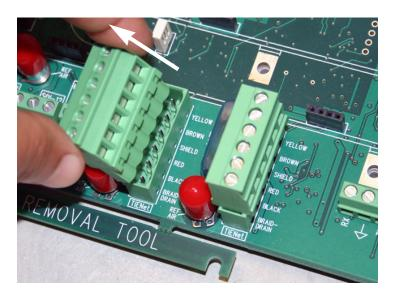
Figure 2-5 TIENet Device terminal strips
