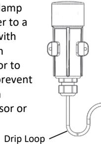
The U23-001 or U23-001A logger must be mounted horizontally. If the U23-001 or U23-001A logger is being deployed in a solar radiation shield, it must be mounted horizontally.
