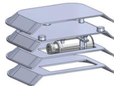
The external sensor for a U23-002 or U23-002A logger, must be mounted vertically. If the sensor is being deployed in a solar radiation shield, it must be mounted as shown.
