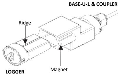
For BASE-U-4 or the HOBO Waterproof Shuttle, firmly insert the optical end of the base station into the D-shaped end of the coupler, and make sure that the ridge on the logger is aligned with the groove in the coupler. If you are using the HOBO Waterproof Shuttle, briefly press the coupler lever to put the shuttle into base station mode.
