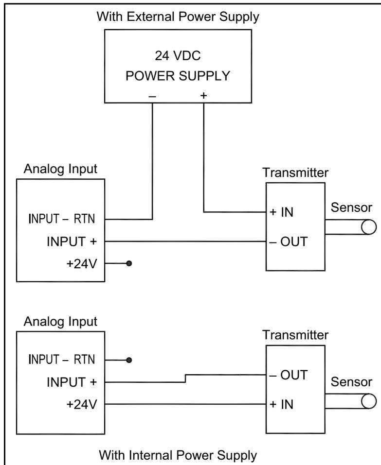
**Figure 5: Analog Input Wiring Diagram**
