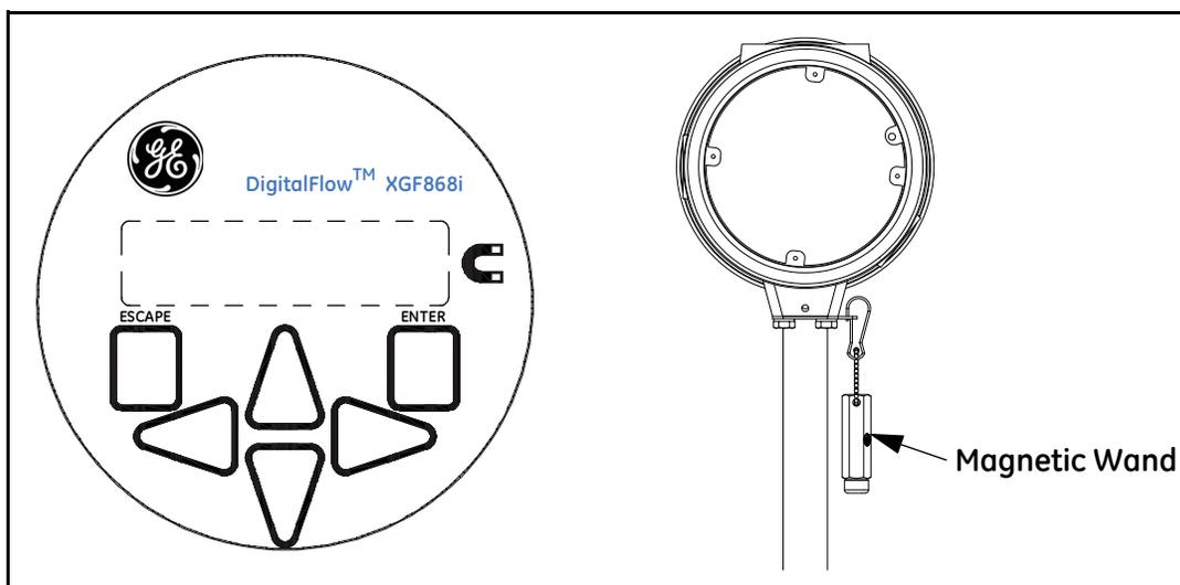
Figure 13: XMT868i Magnetic Keypad and Wand
