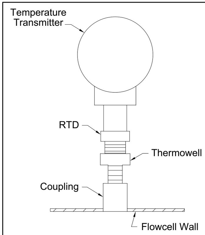
Figure 2: Typical Temperature Transmitter Mounting
