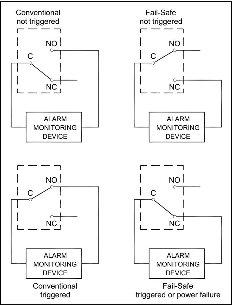
Figure 4: Conventional and Fail-Safe Operation
